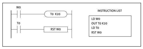
This example will maintain the W0 ON state for a time of 2 secs ( $20 \times 100$  ms). After this time, W0 will be set to OFF.
