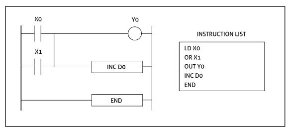
In this program, **LD X0** and **LD X1** are contact instructions and **OUT Y0**, **INC D0** and **END** are coil instructions. Coil instructions are always shown aligned to the right in a ladder diagram. X0, X1 and Y0 are bit devices, D0 is a word device. The lines can be seen as signal wires spreading the condition signal.
