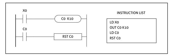
The above example will count 10 pulses in X0 input. When the count is reached, the counter is reset to start again.
